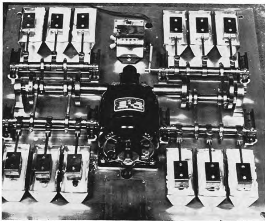
FIGURE 1. PHOTOGRAPH OF COLLEGE OF PHYSICIANS AND SURGEONS ABRASION MACHINE, SHOWING MOTOR, WITH BUILT-IN REDUCING GEAR, ECCENTRIC SHAFTS, BRUSH HOLDERS, AND CUPS, COUNTING AND SWITCH MECHANISM, ETC.
